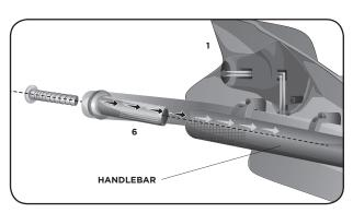
• Install the expander bolts (6), and fix the hand guard to the handlebar.
