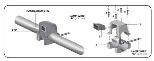
• Secure to the switch (9) with the lamp wires to the switch body (8) and mount to the handlebar • Secure to the Silver with the 4 screws (2).
