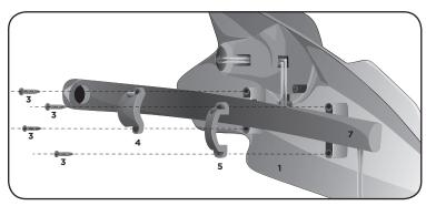
• Fix the hand-guard on the mounting bars (7) through the collars (4/5) and secure with screws (3). (Please note the direction of the shaped collars.) The wire should be installed in the groove in the mounting bar.
