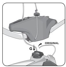
6. Remove the breather pipe from the main tank and replace this with the syphon kit provided (G). Your tank will now breath through your new handlebar tank and fuel will syphon as you ride into your main tank.
