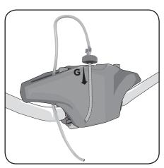
5. Fill up bike tank and also the handlebar tank, assemble the cap making sure the syphon tube goes to the bottom of the fuel tank.
