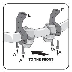
To fix the bracket on the handle-bar without closing the screws firmly.
