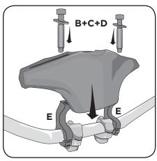
**3.** Position the additional tank over the handle-bar and brackets and secure with the bolts provided.
