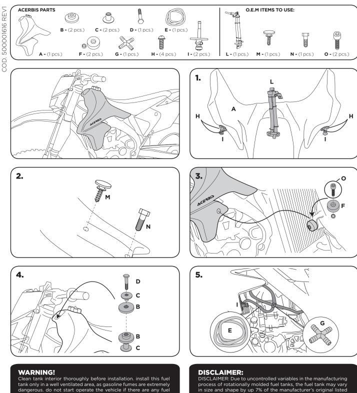
tank only in a well ventilated area, as gasoline fumes are extremely dangerous. do not start operate the vehicle if there are any fuel leaks! acerbis recommends that installation be done by licensed mechanic. read all instructions first before beginning installation.
