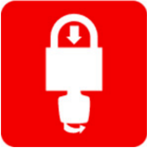
Key-retaining Lock retains key until locked
