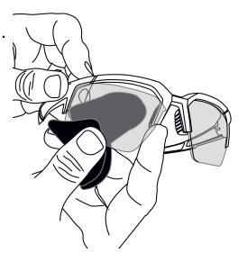
3. Once the lens is inserted in the channel gently apply pressure on the lens with your fingers while applying pressure with your thumb on the frame. This will cause the remaining lens mounting tab to "pop" into place.
