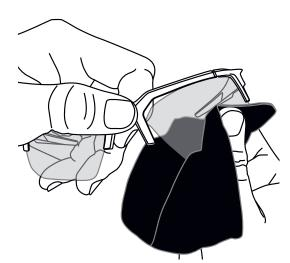
2. Once the inside lens mounting tab is free, continue pivoting the lens until the mounting tab on the end of the lens easily releases from the frame.
