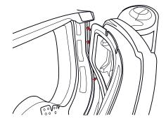
3. Install a new roll of film into the left side canister. Make sure the top of the axle is slot side up.
