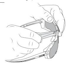
2. Slide the tool under the nose bridge, gently push forward to catch and release the tab that locks the lens latch onto the bottom inside of the nose bridge.
